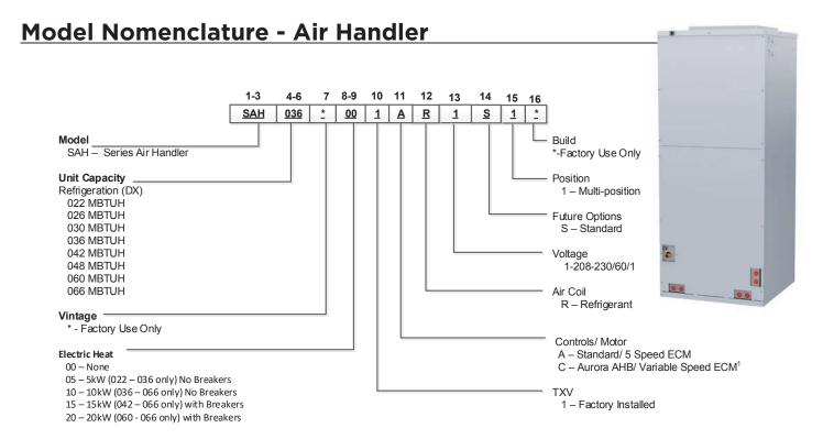
Note: To field convert the SAH to bottomflow air discharge, the SAHBCK kit must be ordered. Note: Air flow on the 060 and 066 units in the horizontal configurations should be limited to 1900 cfm in cooling mode, or condensate blow off may occur.
