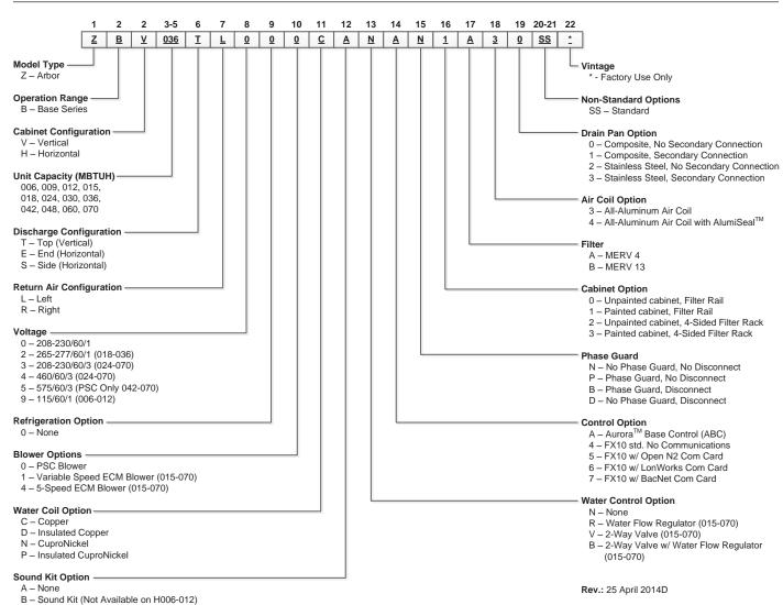
Note: Phase Guard Only Available on 208-230/60/3, 460/60/3, and 575/60/3 50VA Transformer with Aurora and 75VA Transformer with FX10
