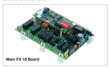
The FX10 is a microprocessor based control that not only monitors and controls the heat pump but also can communicate any of this information back to the building automation system (BAS). This means that not only does the control monitor the heat pump at the unit you can also monitor and control many the features over the BAS. This clearly puts the FX10 in a class of its own.
