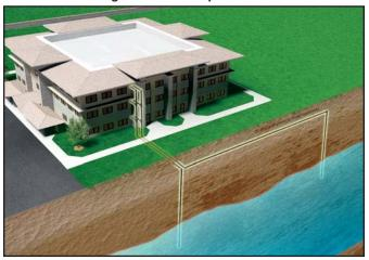
Closed Loop/Ground Water Plate Heat Exchanger
