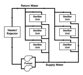
comfortable environment for all building areas. Excess heat can be stored for later utilization or be added or removed in one of three ways; by ground-source heat exchanger loops: plate heat exchangers connected to other water sources, or conventional cooler/boiler configurations. Your GeoStar representative has the expertise and computer software to assist in determining optimum system type for specific applications.
