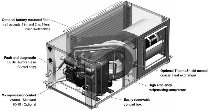
Four blower deck options are available. Factory or field conversion option of end or side discharge using switchable access panels and a factory only option of true left or right return air coil.
