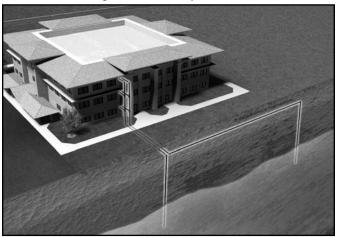
Closed Loop/Ground Water Plate Heat Exchanger
