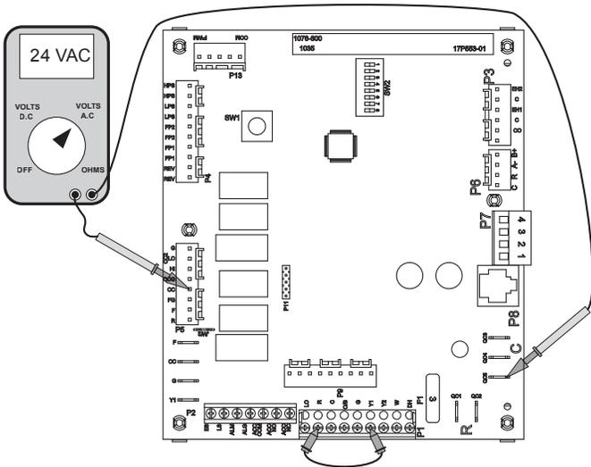
With the AID Tool go to the “Thermostat Inputs” Menu under “Diagnostics” and over-ride the “Y1” input to ON. If an AID Tool is not available remove the P1 connector to disconnect the thermostat from the board and place a jumper wire between “R” and “Y1” as shown. Apply power and put the board into test mode by holding SW1 for 2-5 seconds, the green LED will begin a slow flash. Connect your Volt meter leads to “CC” and “C”. After 1 minute the reading should be between 18 and 30VAC. If you have
