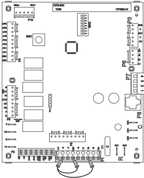
How it works: The condensate sensor is a three part system: a wire, air coil, and water in the drain pan. The wire (spade terminal) and air coil act like a normally open contact and the water acts as the switch. When water in the drain pan fills up and touches the spade terminal, the unit will fault on condensate.
