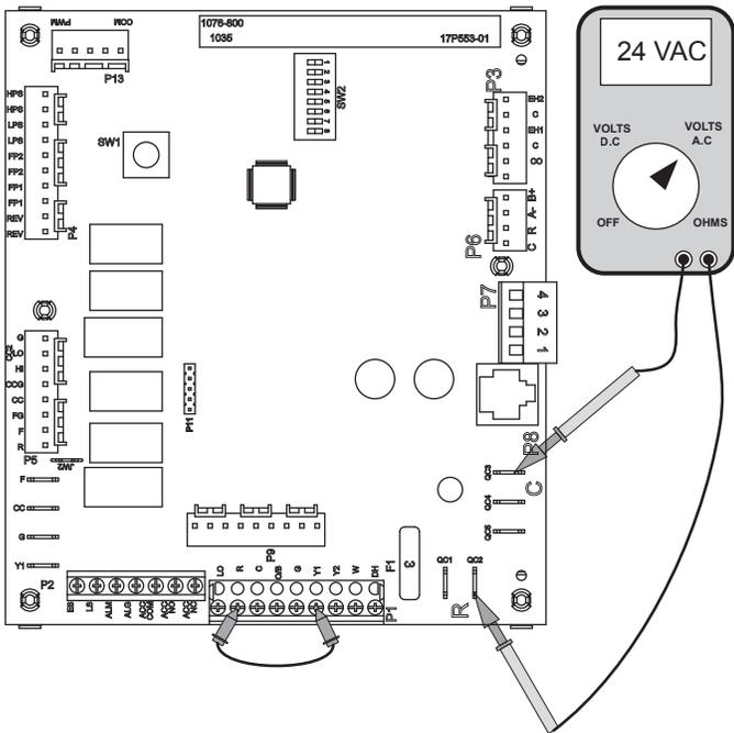
With power applied to the unit connect your Volt meter leads to “R” and “C” on the control board where the yellow and black/white transformer wires connect. The reading should be between 18VAC and 30VAC.
