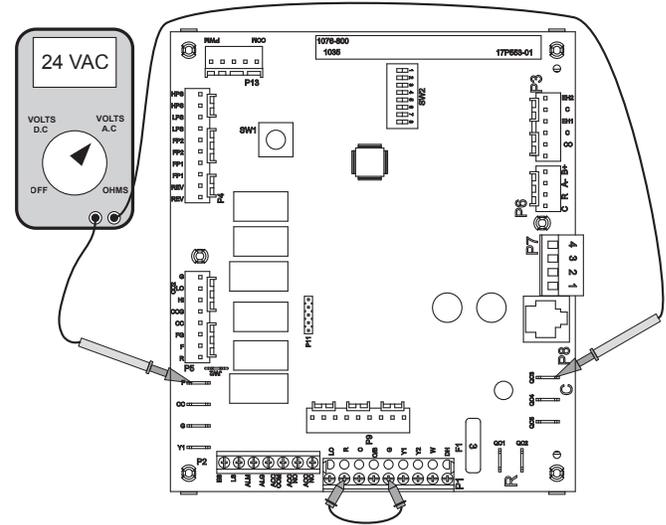
With the AID Tool go to the “Thermostat Inputs” Menu under “Diagnostics” and over-ride the “G” input to ON. If an AID Tool is not available remove the P1 connector to disconnect the thermostat from the board and place a jumper between “R” and “G” as shown. Put the board into test mode by holding SW1 for 2-5 seconds. The blower will come on and run in the “G” speed setting. To check the enable signal to the motor, measure 24VAC between the F and C terminals.
