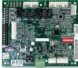
Aurora uses the Modbus communication protocol to communicate between modules. Each module contains the logic to control all features that are connected to the module. The Aurora 'Base' Control (ABC) has two Modbus channels. The first channel is configured as a master for connecting to devices such as a communicating thermostat, expansion board, or other slave devices. The second channel is configured as a slave for connecting the Aurora Interface Diagnostics Tool (AID Tool).
