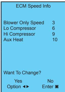
current ECM settings. It allows the technician to enter the setup screens to change the ECM settings. Change the highlighted item using the ◀ and ▶ buttons and then press the ◻ button to select the item.
