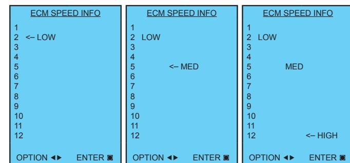
After the high speed setting is selected the AID Tool will automatically transfer back to the ECM Setup screen.
