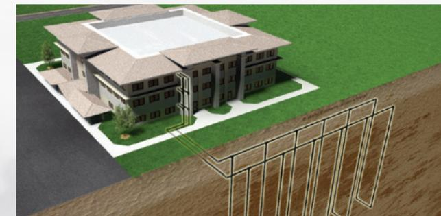
**VERTICAL LOOP:** The ideal choice when limited land surface is available. Well-drilling equipment is used to bore the 75 ft. to 300 ft. deep, small-diameter holes that will accommodate the loop.
