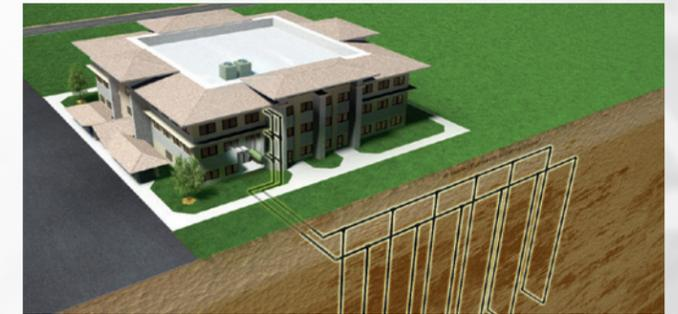
**HYBRID LOOP:** Combines boiler tower and geothermal loop technologies to achieve optimal efficiencies, while meeting the challenges of both loop field space and budget constraints.
