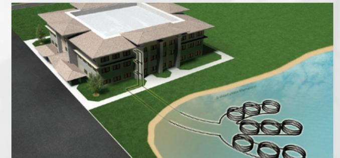
**POND LOOP:** Very economical to install when an adequate body of water is available, because excavation costs are virtually eliminated. Coils of pipe are simply placed on the bottom of the nearby pond or lake.
