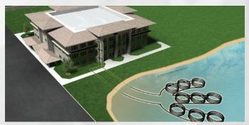
**POND LOOP:** Very economical to install when an adequate body of water is available, because excavation costs are virtually eliminated. Coils of pipe are simply placed on the bottom of the nearby pond or lake.
