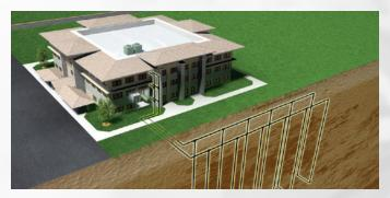
**HYBRID LOOP:** Combines boiler tower and geothermal loop technologies to achieve optimal efficiencies, while meeting the challenges of both loop field space and budget constraints.
