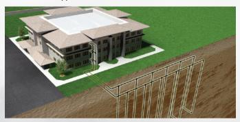
**VERTICAL LOOP:** The ideal choice when limited land surface is available. Well-drilling equipment is used to bore the 75 ft. to 300 ft. deep, small-diameter holes that will accommodate the loop.
