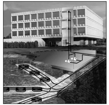
• Closed Loop/Ground-Source Surface Water Systems also utilize the stable temperatures of Surface Water to maintain proper water source temperatures for Aston Series extended range heat pump systems. These systems have all of the advantages of horizontal and vertical closed loop systems. Due to the extended loop temperatures, AHRI/ISO 13256-1 Ground Water or Ground Loop Heat Pumps are required for this application.
