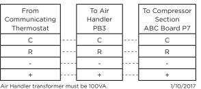
Air Handler transformer must be 100VA.
