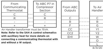
Non-Communicating Thermostat Control Option C Field low voltage point to point wiring:
