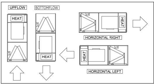
FIGURE 3: Typical Installation
