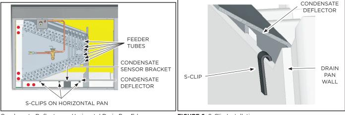
Condensate Deflector on Horizontal Drain Pan Edge
