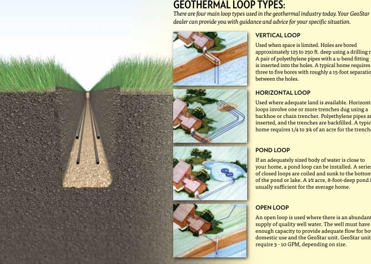
Used when space is limited. Holes are bored approximately 125 to 250 ft. deep using a drilling rig. A pair of polyethylene pipes with a u-bend fitting is inserted into the holes. A typical home requires three to five bores with roughly a 15-foot separation between the holes.
